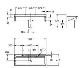
Wall mounted washtroughs with tap ledge and optional rear splashbacks incorporating manual or electronic self-closing water controls, manufactured from 1.2 mm thick stainless steel. 1200 mm Washtrough with tap ledge for 2 users.
