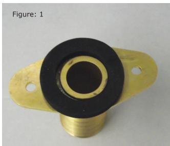
Figure: 1 Put seal on the end of waste fixing and place over waste outlet at rear of basin. See Figure 2.
