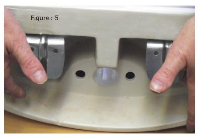
Figure 5: Fasten wall brackets to cavity wall firmly using silicone sealant along rear of basin for extra strength. Slide basin over wall brackets. Run bead of silicone around rear of basin to finish.
