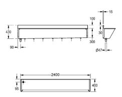
SATURN Scrub up trough, grade 1.4301 (304) stainless steel with satin finish, material thickness 1.5mm. Supplied with a convential waste outlet in the base of the trough and shroud to cover pipework. Fixed to the wall using joggle strips supplied. Manufactured in accordance with HTM64/HBN 00-10 Part C standards.
