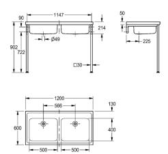
A double bowl sink manufactured from 1.2 mm thick, grade 1.4301 (304) stainless steel, satin polish finish. The sink top is turned down on all four edges and incorporates a wet area recess. The bowls are prepared for a 38 mm waste outlet.
